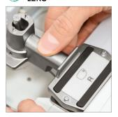
FIT SILICONE SEAL TO INNER BEVEL
